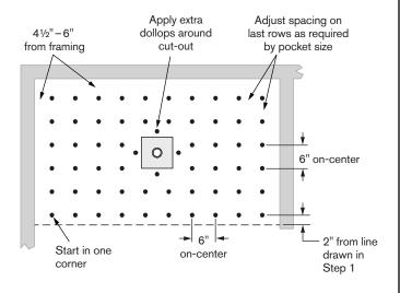
3 TIP SHOWER UP into position. Make sure it aligns with line drawn in Step 1. Avoid stepping in shower until adhesive has cured.
