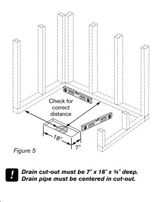
Have a plumber prepare drain pipe to receive the drain; the pipe must be centered in the 7" x 18" x 3/4" deep cut-out.
