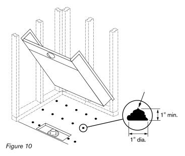
Epoxy supplied by Bestbath is intended for adhering the pan to the subfloor. It should not be used for leveling the subfloor. If the subfloor does not meet stated requirements, please use an appropriate product (not supplied) to level the subfloor prior to installation.
