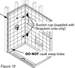
For SnapJoint Walls ONLY: With a suction cup on lower back wall panel, pull it firmly forward until back and side walls are pulled together. You will hear a series of clicks as the panel locking clip engages. Repeat with upper panel. (Figure 13)
