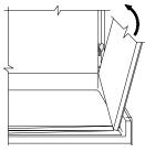
With walls firmly pushed down and front edge of side wall aligned with front edge of pan, screw through side wall flanges into framing.
