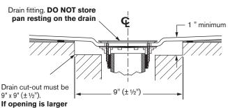
it must be adjusted to 9" x 9" with structural material (such as wood, cement, etc.) to prevent flexing.
