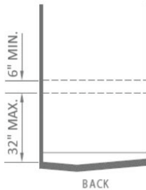
(c) GRAB BAR REINFORCEMENT FOR ADAPTABLE SHOWERS
