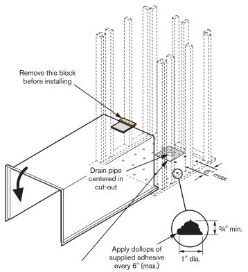
Drain cut-out must be 9" x 9" and 1" deep.
