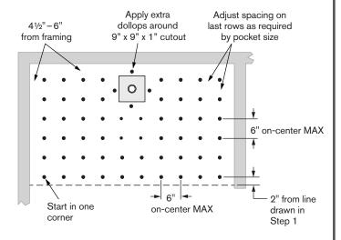
TIP SHOWER UP into position. Make sure it aligns with line drawn in Step 1. Avoid stepping in shower until adhesive has cured.
