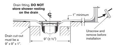
If opening is larger it must be adjusted to the required cut-out with structural material (such as wood, cement, etc.) to prevent flexing.
